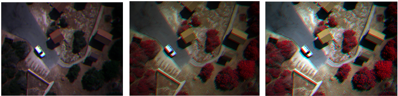
Figure 14: On the left is the rgb image, in the middle is the result when the 4-3-2 band combination (when the 4th band is the NIR) applied on the left image. The right image has been resulted after the linear stretch has been applied on the middle image.
