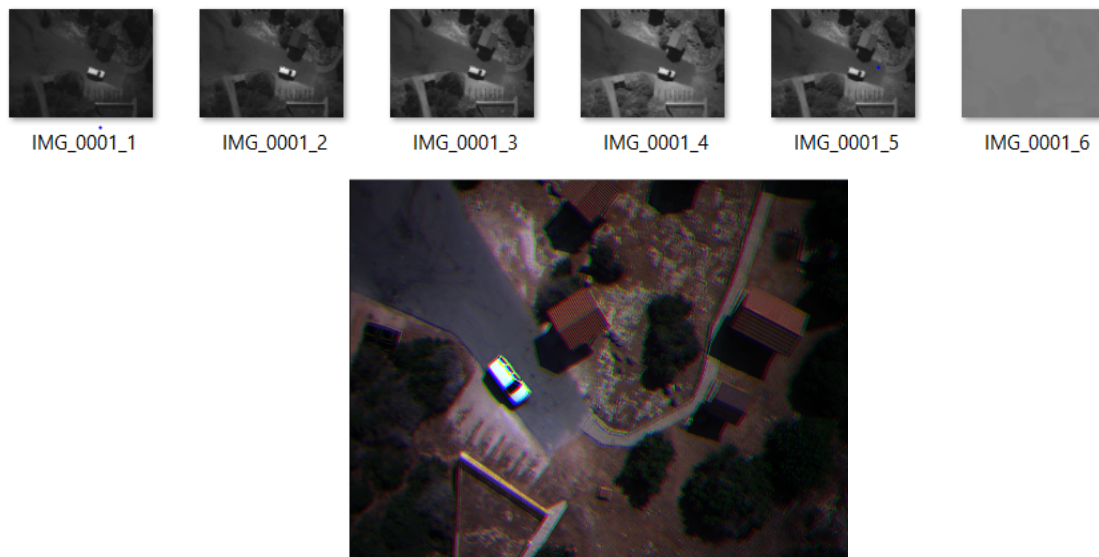
Figure 16: The example of the image stacking for the IMG_001. The 6 bands (blue, green, red, red edge, NIR, thermal) are stacked together and the result of this procedure is a multispectral image.
