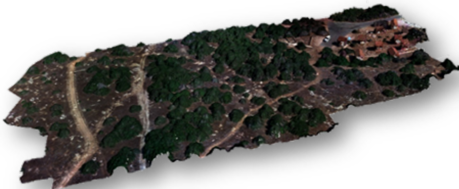
Figure 19: The 3D model which has been resulted after the implementation of different photogrammetric techniques on UAV imagery dataset.
