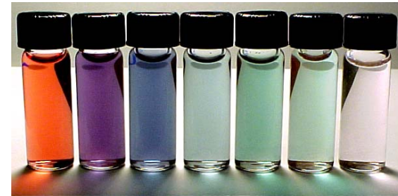
Vial on the left has solid gold colloids. Others have colloids with metal nano-shells with decreasing thickness. Vial on left absorbs IR
