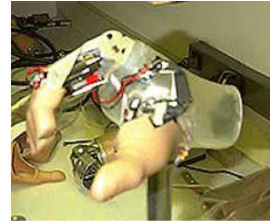
THE CIRCUITRY OF A MYOELECTRIC HAND Courtesy : Inventors.About.com
