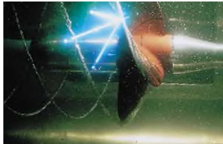
Measurement of flow around a ship propeller in a cavitation tank
