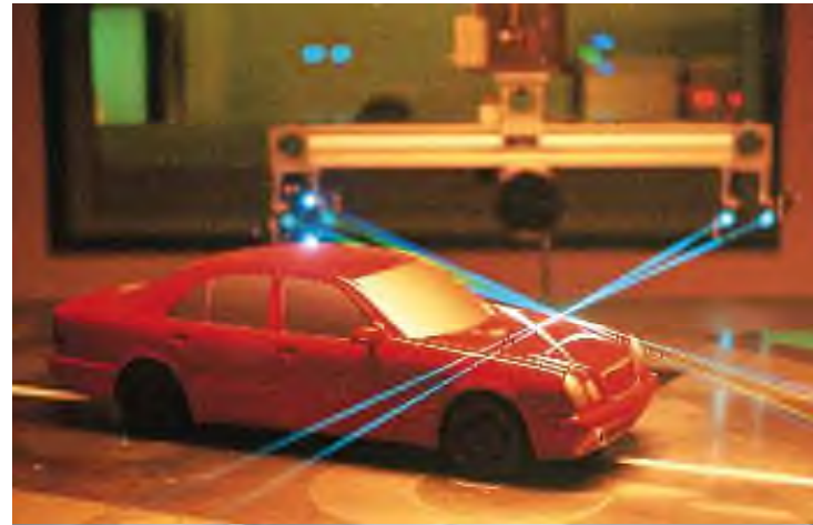
Measurement of flow field around a 1:5 scale car model in a wind tunnel (Photo courtesy of Mercedes-Benz, Germany)
