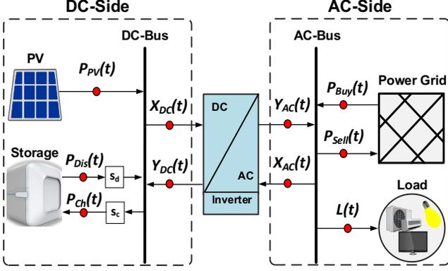
Figure 3. Equivalent model of the system.
