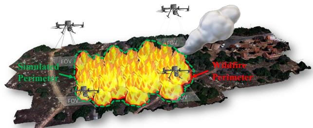
Fig. 1. The proposed multi-UAV system for wildfire perimeter monitoring that integrates the UAVs' sensing capabilities and a wildfire propagation model.
