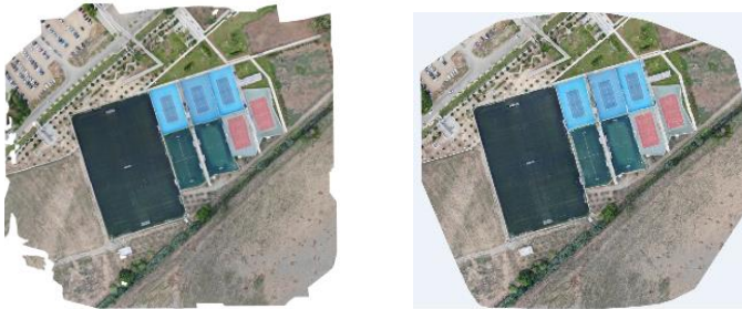
Fig. 9. The above 4 orthophotos have resulted by the end of the 1st experiment. On the 1st row are presenting the two orthophotos created by the Dataset A. On the left is the orthophoto created by the Agisoft Metashape and on the right is the orthophoto created by the same dataset by the OpenDroneMap. On the 2nd row, are presenting the orthophotos created by the two software, having as input the Dataset B
